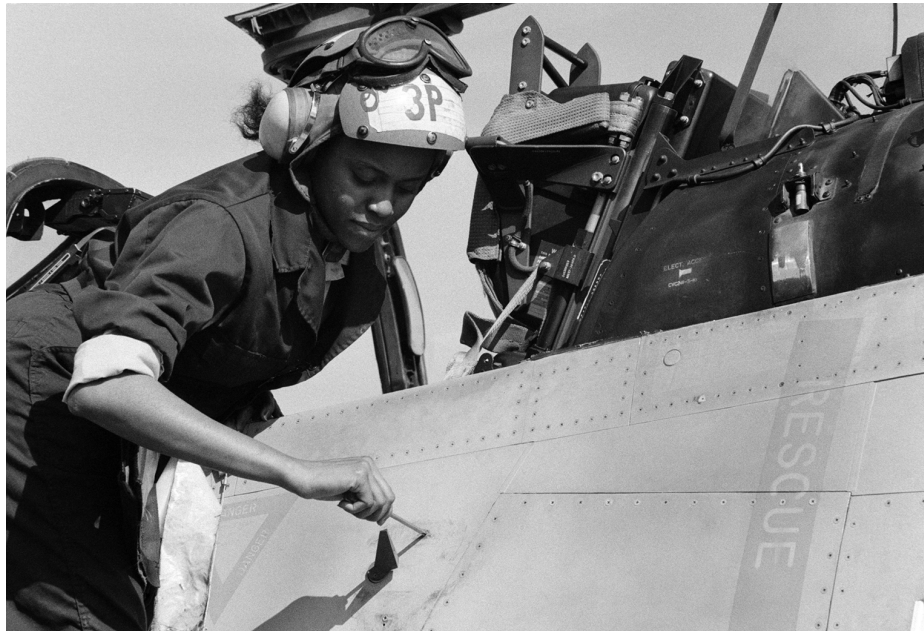
NAID: 6441492 JO3 Cyndi Reilly Naval Air Station, Lemoore, Calif....AIRMAN Ora Howard, plane captain, performs a routine maintenance inspection on an A-7 Corsair II aircraft.
